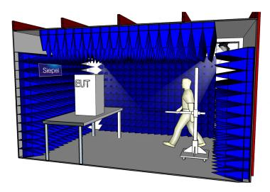
The Ares 1P is designed to perform emission and immunity tests on military and aeronautic devices. The design of the structure is optimised for maximum performances, in minimum space. The chamber and its absorbers are manufactured by SIEPEL.
