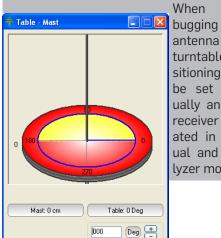
When dethe antenna and turntable positioning can be set manually and the receiver operated in Manual and Analyzer modes.
