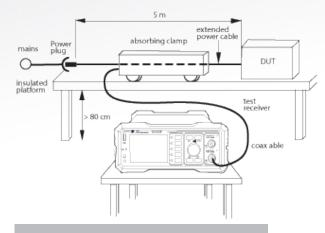
Radiated power measurement set-up with absorbing clamp
