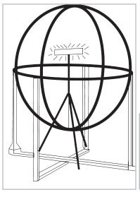
Radiated emission measurements of luminaries by means of the Loop Antenna according to CISPR15/ EN 55015.
