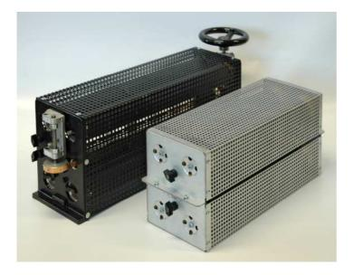
This variable dummy load is used for the compensation of the power current in the measurement setup according to MIL-STD461, CS101, as shown in figure A-8, page 215 of MIL STD 461-F.
