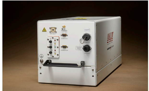
CPI 150 W K-band TWTA, model VZK2791J1.
