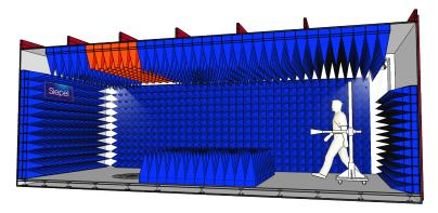
The Hera 3P is designed to perform pre-compliance emission and full compliance immunity tests at 3m distance on commercial equipment. The design of the structure is optimised for maximum performances, in minimum space. The chamber and its absorbers are manufactured by SIEPEL.
