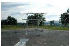
NEMP test system according to MIL STD 461E - RS105 Marx pulse generator 230 kV, rise time 2.3 ns / duration 23 ns with 3.6 m high radiation line
