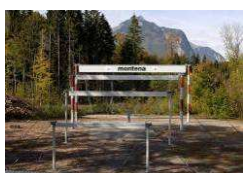
NEMP test radiation for tests according to MIL STD 461E - RS105 Marx pulse generator 800 kV, rise time 2.3 ns / duration 23 ns with 9 m high radiation line
