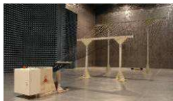
NEMP test system according to MIL STD 461E - RS105 Marx pulse generator 120 kV, rise time 2.3 ns / duration 23 ns with 2.7 m high radiation line
