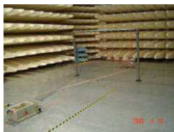
NEMP test system according to MIL STD 461E - RS105 loading voltage 80 kV rise time 2.3 ns / duration 23 ns with 1.8 m high radiation line
